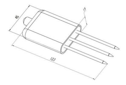
Equipment size drawing (unit: mm)
